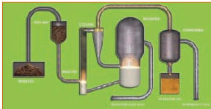
The Envergent Rapid Thermal Processing (RTP) system
