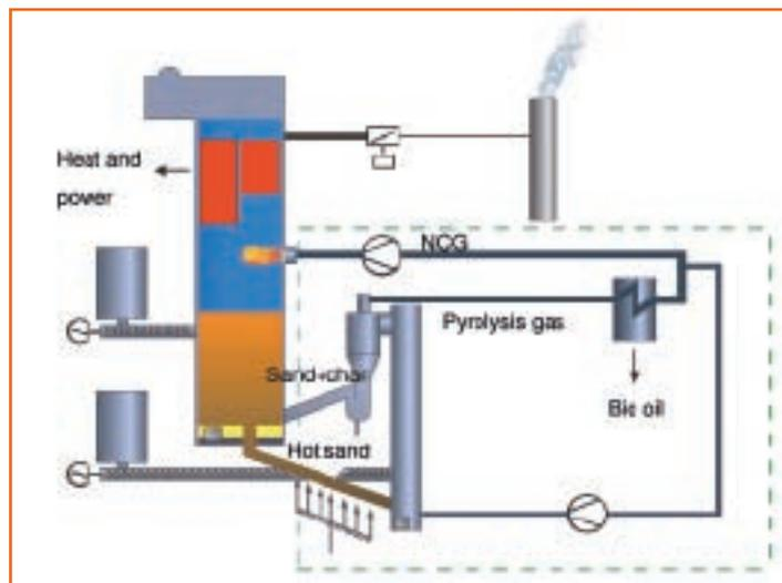
A Metso fluid bed boiler used in a heat and power plant integrated with a pyrolysis system
