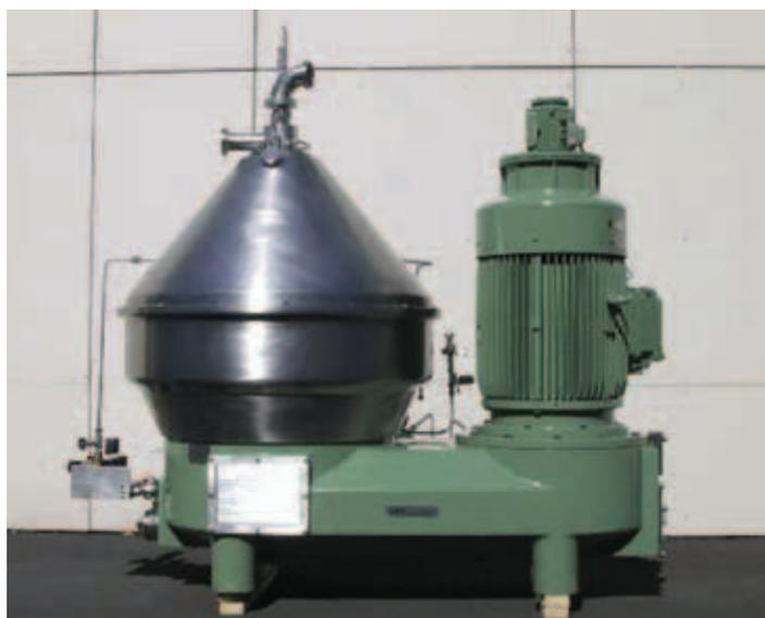
A small Westfalia disc centrifuge for biodiesel, supplied by Kyte Centrifuge
