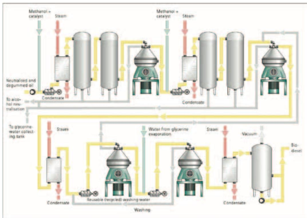
Schematic of a Westfalia centrifuge equipped biodiesel production plant
