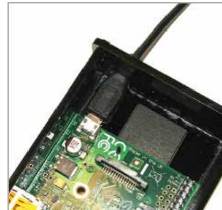
▲ The extended case keeps the SD card secure
