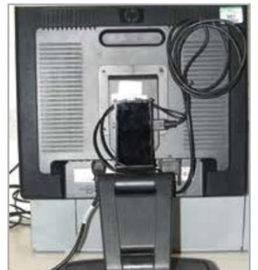
▲ Raspberry Pi mounted on the rear of the monitor and cables coiled up neatly
